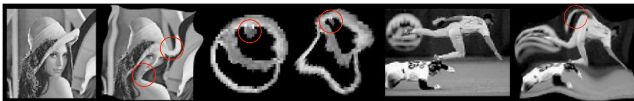
Figure 5.12: Pairs of images used in the synthetic experiments (Lena, heart, baseball player). Each left image is a fixed image, each right side is a moving image generated with a random deformation of at most 25 pixels (difficulties in red). These transformations provide our ground truth.
