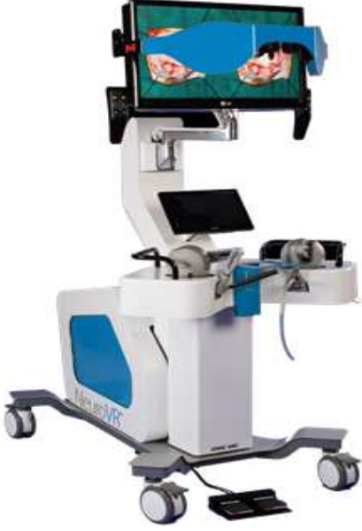
Figure 2: The virtual reality neurosurgery simulator, NeuroTouch, at the National Research Council of Canada.
